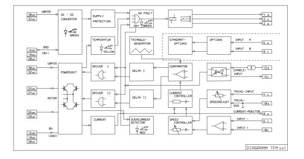
A) The TFMxx1 has a **Built-in Power Supply** which converts the intermediate circuit voltage to an **internal power supply voltage**. Therefore the controller **never needs an external power supply**. The function of the internal power supply **includes also checking an monitoring** (LED) the whole functions of each TFMxx1. Faults are **monitored** by a Failure Output (relay) and several LED's on the front panel.
